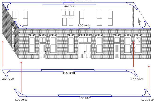
Glue provided corner supports (LCC 70-00) into inner corners as shown on the diagram. It is recommended to strengthen the elevations with provided LCC 70-01. Glue 3 full length pieces from LCC 70-01 together with one overlapping on top. Then glue them to the backs of elevations. If the model is going to be glued to baseboard promptly it is possible to omit all of the above supports altogether.
